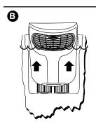
Lift upward on filter cover to remove it from the mating retaining clips. Then tilt forward to access filter cartridges.
