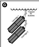
Submerge both filter cartridges in spa. Tilt threaded end upward to remove trapped air bubbles, then keep cartridges submerged to prevent air entrapment during installation (step H).
