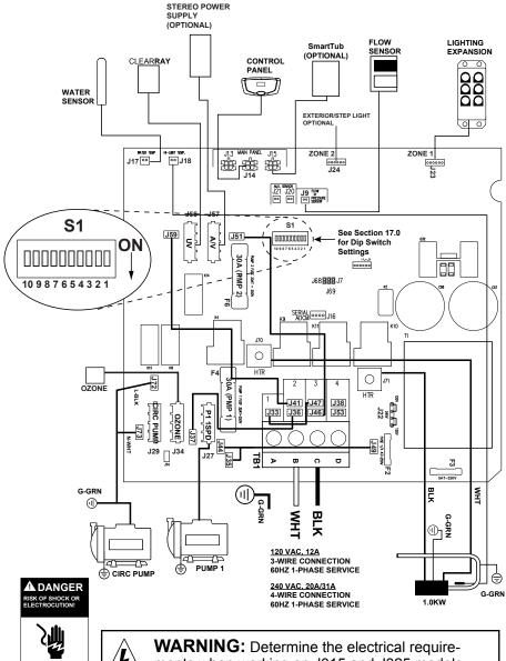
Turn power off before servicing. This task should only be performed by a qualified technician. **WARNING:** Determine the electrical requirements when working on J315 and J325 models. These models are available in a dedicated 240V 60Hz or 120V/240V 60Hz convertible configuration.
