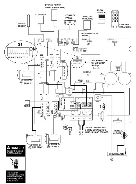
**16.2 J-315** and **J-325 3-Wire 240V 60Hz Dedicated Power Models** This wiring diagram is used for a 3-Wire 240V 60 Hz dedicated power models.
