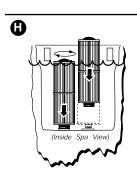
Place each cartridge back into skimmer well, then rotated each cartridge handle clockwise to thread back into wall fitting. DO NOT OVERTIGHTEN!
