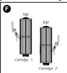
If used, remove the chemical feeder as instructed prior to rinsing the filter cartridges. Rinse debris from filter pleats on each cartridge using a garden hose and high pressure nozzle. Start at the top and work downward towards handle. Repeat until all pleats are clean.
