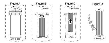
To ensure optimum performance, clean skimmer basket and filter cartridge once a month or as necessary, depending on use.
