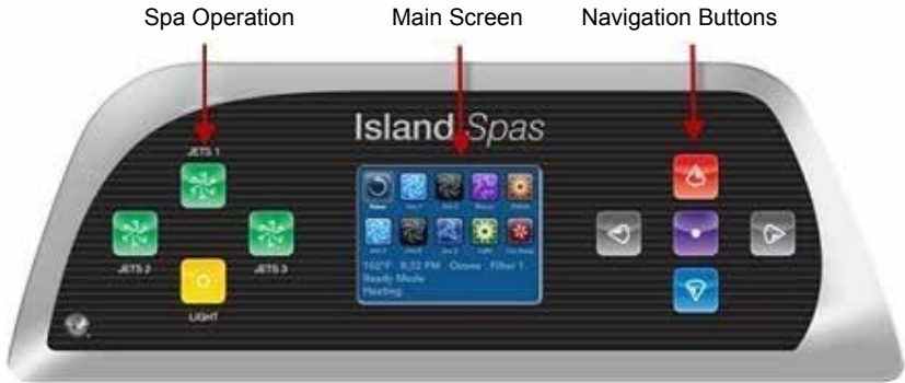
Island Spas 3 Pump Topside
